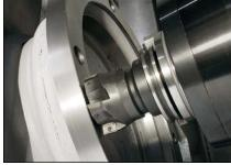
The EC-1600 and EC-1600YZT are equipped with a 6000-rpm geared-head 50-taper spindle that provides 450 ft-lb of torque for heavy cutting. For high-speed cutting, a 10,000-rpm gearedhead spindle is available.
