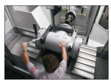
The EC-1600 and EC-1600YZT are available with a full 4th-axis rotary platter integrated into the T-slot table to provide access to four sides of a part or tombstone. The 30" platter handles parts and fixtures up to 10,000 lb.
